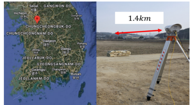
FIG. 6. Location of the measurement site and scintillometer setup over a 1.4 km path.
