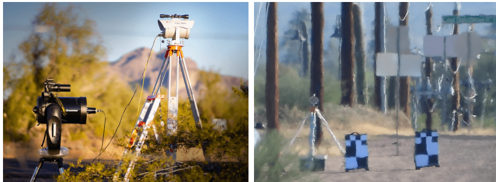
(a) Nikon camera on top of telescope (left side) and scintillometer (right side) (b) A cropped portion of the original images containing target
